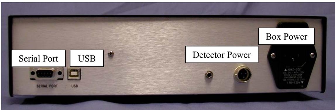
**Figure 6.** Rear of electronics box. The communications ports are on the left. Use only one.
