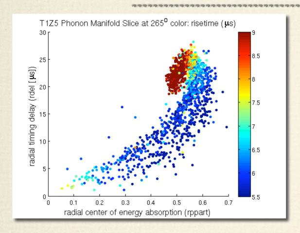
New metric compares start times of inner 3 channels to the start time of outer channel, breaks degeneracy.
