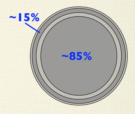
Inner Channel: ionization measurement Outer Channel: fiducial volume
