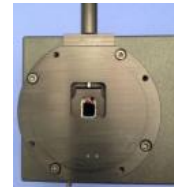
Fig. 1 Circular Flange on back of AMPLIFIER MODULE
