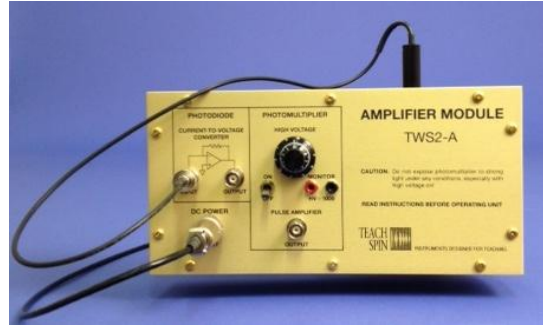
Fig. 4 AMPLIFIER MODULE with shutter to photomultiplier closed.
