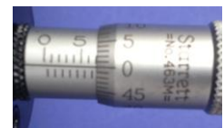
Fig 6. A reminder of how to read the micrometer
