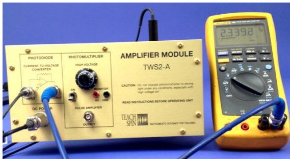
Fig. 3 AMPLIFIER MODULE with I-to-V converter connected to multimeter
