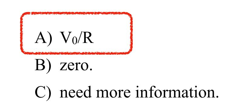
Immediately after the switch is thrown closed, the current is  $V_0/R$ . It decreases from this value to zero exponentially, with a time constant equal to RC.
