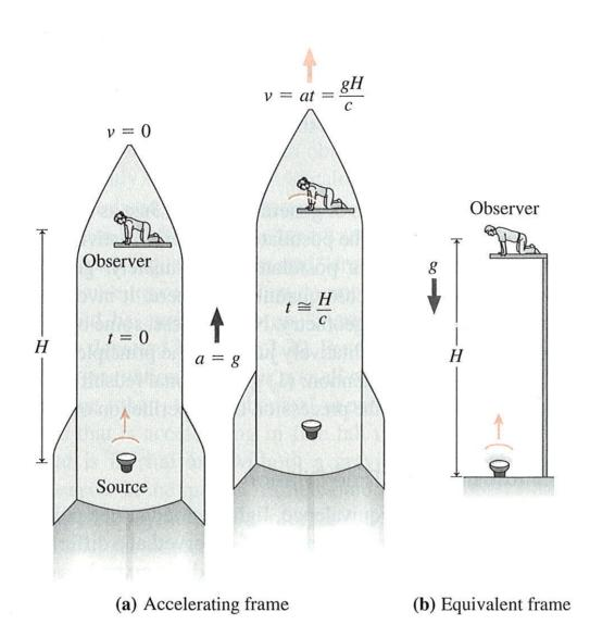
$$\Delta t_{lower} = \Delta t_{higher} (1 - \frac{gH}{c^2})$$
