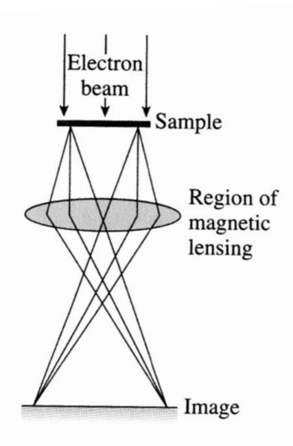
**Basic principle:** A beam of electrons is accelerated through a potential difference. After passing through a series of "lenses", the electron beam produces an image on a screen.
