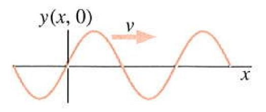
After one wave cycle, the cycle repeats. The repetition rate is the frequency.
