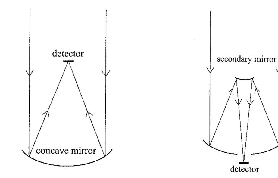
Detector at prime focus Aperture is primary mirror.
