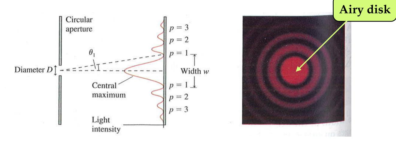
Light waves from outside must pass through a circular lens. The performance limit of optical instruments is determined by the diffraction of the circular openings through which the waves must pass.
