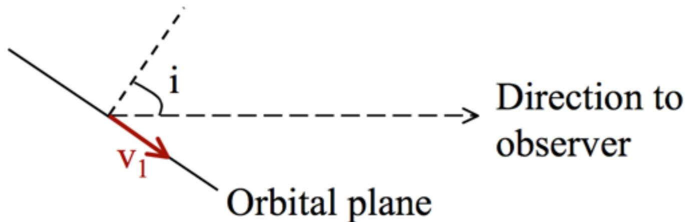
$$|v_{1\text{obs}}| = |v_1| \sin i$$
