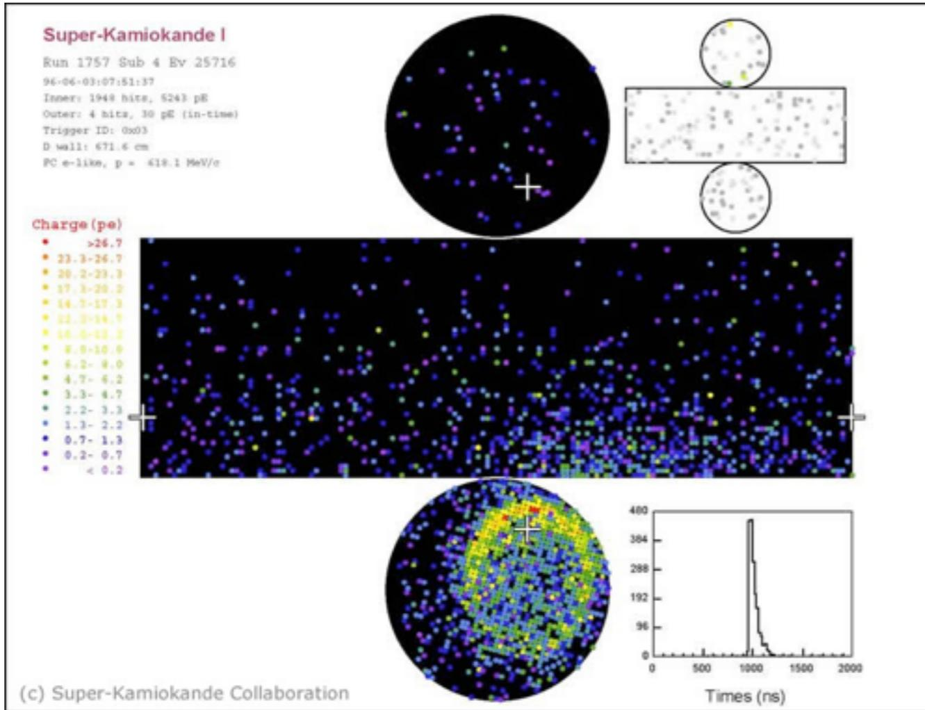
The emitted electron from a  $\nu_e$  interaction generates an EM shower which produces an image with a fuzzy Cherenkov ring.
