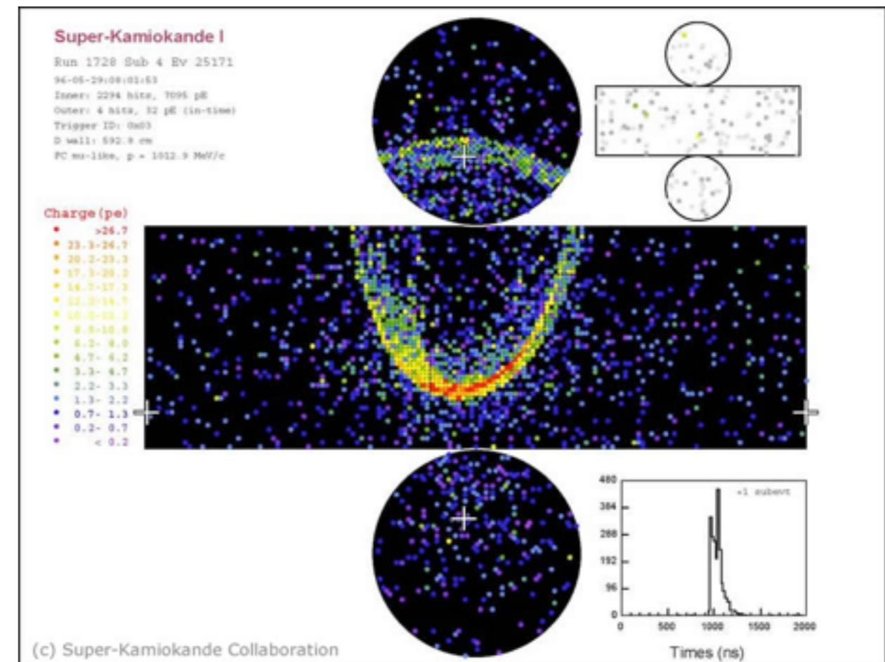
The emitted muon from a  $\nu_\mu$  interaction generates an image with a crisp Cherenkov ring.
