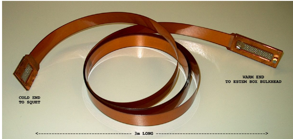
Figure 3.12: The cold end of a stripline connects to a SQUET and the warm end of it connects to the E-box. It transfers the collected signals from the cryogenic region to the room-temperature electronic system.
