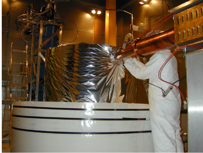
Figure 3.10: This photo is to show the assembly of shielding layers near the cryogenic region at Soudan site.
