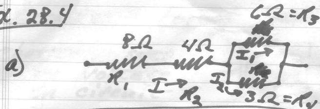
$$R_{\text{eq}} = R_1 + R_2 + \frac{R_3 R_4}{R_3 + R_4}$$
