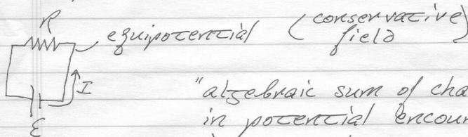
"algebraic sum of changes in potential encountered in a complete traversal of the circuit must be zero."
