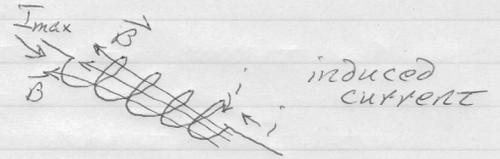
We can increase inductance by multiplying # loops, as shown for coil above.
