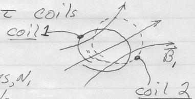
Coil 1 has current which sets up magnetic field,  $B_1$
