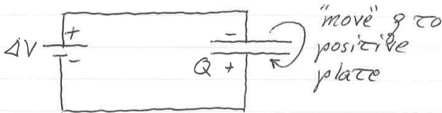
To understand the energy stored, need to consider work done to put charge on capacitor
