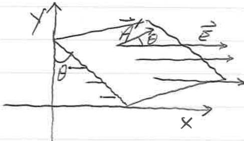
$$\begin{aligned}\underline{\underline{\Phi_E}} &= \underline{\underline{\vec{E} \cdot \vec{A}'}} \\ &= \underline{\underline{EA' \cos \theta}}\end{aligned}$$
