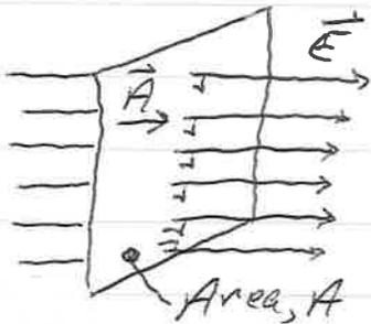
$$\begin{aligned}\underline{\underline{\Phi_E}} &= \underline{\underline{\vec{E} \cdot \vec{A}}} \\ &= \underline{\underline{EA}}\end{aligned}$$
