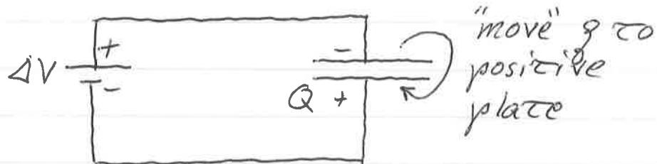
To understand the energy stored, need to consider work done to put charge on capacitor
