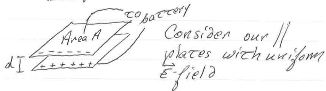
Disconnect the battery & increase separation to  $d'$
