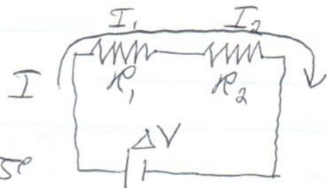
Potential drops  $\Delta V$  divided between resistors
