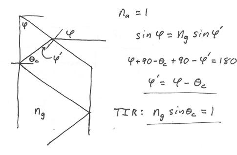
$$\sin \varphi = n_g \sin (\varphi - \theta_c) = n_g \left( \sin \varphi \cos \theta_c - \cos \varphi \sin \theta_c \right)$$
