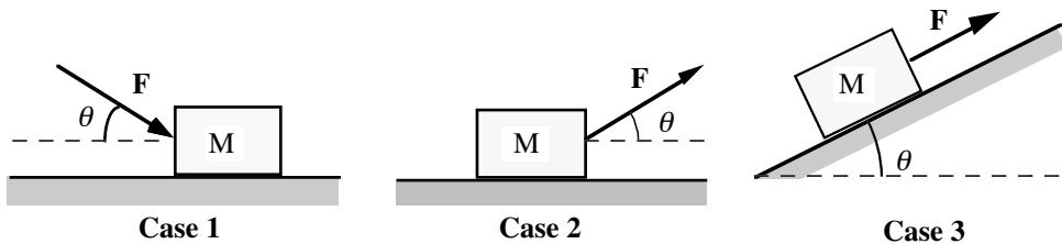
9. In which case will the magnitude of the normal force on the block in the above figure be equal to  $(Mg + F \sin \theta)$ ?
