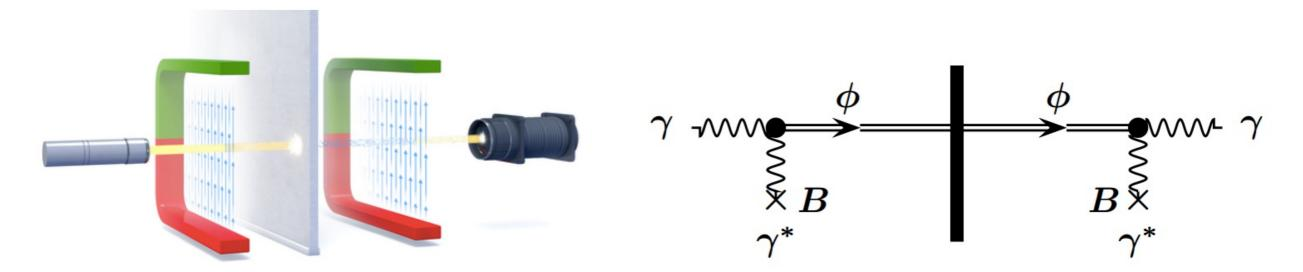
Laser light is shone into a magnetic field. Laser photons can be converted into a WISP in front of a light-blocking barrier (production region) and reconverted into photons behind that barrier (regeneration region).
