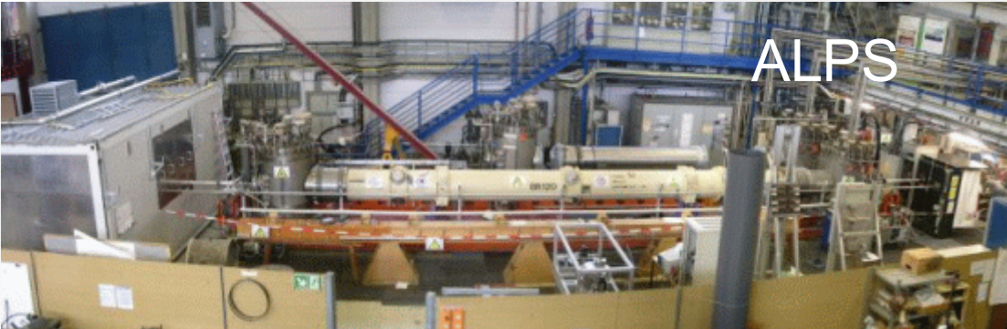
laser shining through a wall in a magnet
