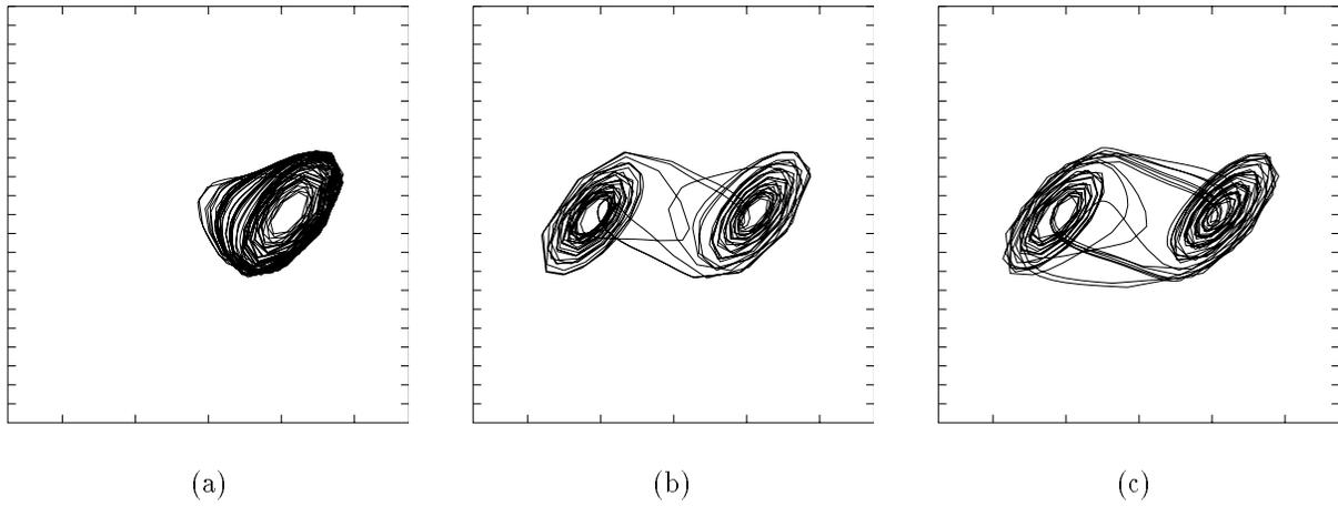
Figure 16: Attractors in Chua's circuit from SPICE 3d2 simulations of the  $C_1$  bifurcation sequence. Horizontal axis  $v_{C_1}$  2V/div; vertical axis  $v_{C_2}$  200mV/div. (a)  $C_1 = 10.1nF$ , Rössler-type attractor; (b)  $C_1 = 9.5nF$ , Double Scroll attractor; (c)  $C_1 = 8.5nF$ , Double Scroll attractor.
