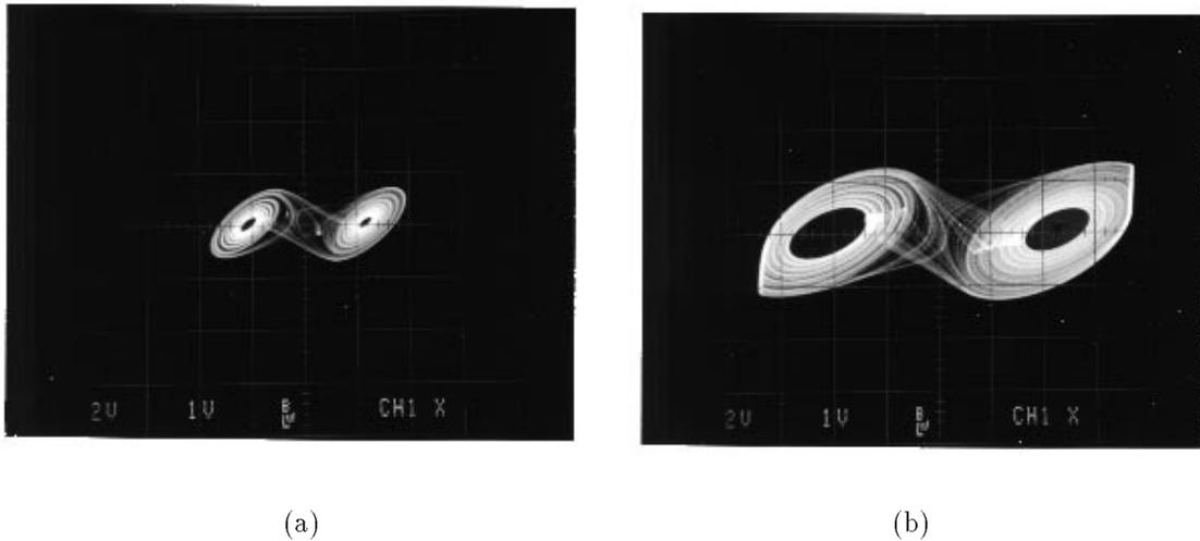
Figure 17: When the attractor is too large, we cannot neglect the effects of the outer regions of the five-segment  $v - i$  characteristic. (a)  $C_1 = 10nF$ : Double Scroll attractor is restricted to the regions of negative slope; (b)  $C_1 = 8nF$ : attractor is distorted by the outer positive-going segments.
