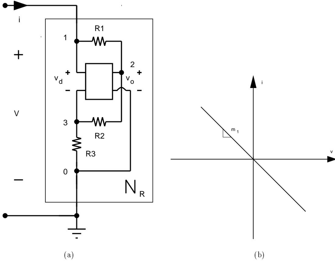
Figure 5: (a) Negative resistance converter using a voltage-controlled voltage source; (b)  $v - i$  characteristic of negative resistance converter using a linear VCVS with linear voltage transfer function  $v_o = Av_d$ . The slope of the  $v - i$  characteristic is given by  $m_1 = \left[ \frac{(1-A)R_2 + R_3}{R_1[R_2 + (1+A)R_3]} \right]$ ; for sufficiently large  $A$ ,  $i \approx -\frac{R_2}{R_1 R_3} v$ .
