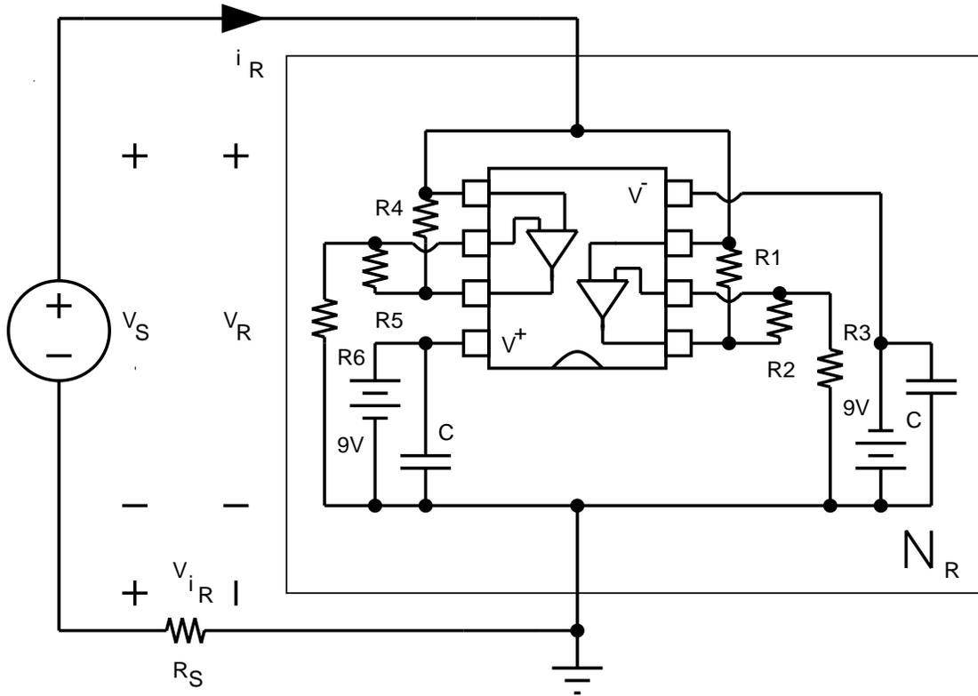
Figure 12: The  $v-i$  characteristic of negative resistor  $N_R$  can be measured by applying a triangular voltage waveform  $v_S$  to the series combination of  $N_R$  and a small current-sensing resistor  $R_S$ . Plot  $-v_{i_R} (\propto i_R)$  versus  $v_R$ . The eight-pin dual op amp package is shown from above in schematic form. The reference end of the package is indicated by a dot or a semicircle (shown here).
