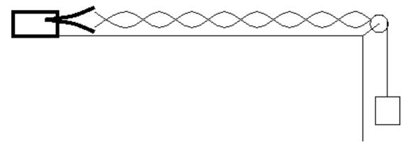
The equation describing standing waves in a string under tension is
