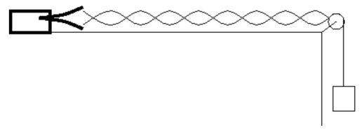
Adding mass to the hanger will change the tension in the string. This will change the wave speed in the string. With the frequency and string length fixed throughout the experiment, we will generate different standing wave modes with different wavelengths. We will measure the wavelengths of the various standing waves and find the relationship between tension and wavelength.
