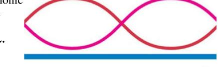
2) For an closed organ pipe, the wave pattern for the lowest frequencies is shown. If L=1 meter, v=340m/s, find the frequency f in Hz. Recall:  $V=f \lambda$ .
