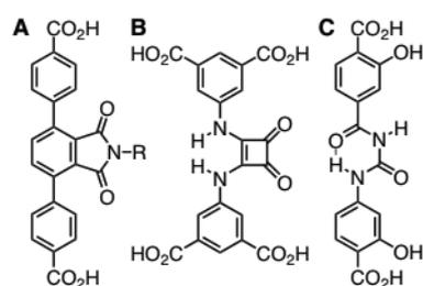
**Fig 2.** Three examples of functionalised MOF struts.
