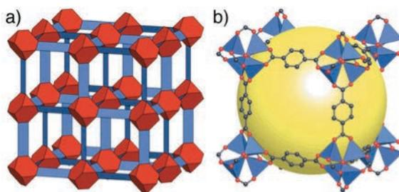
**Fig 1.** a) Schematic MOF diagram showing organic struts connected by clusters. b) One of the many spherical nanopores in MOF-5.
