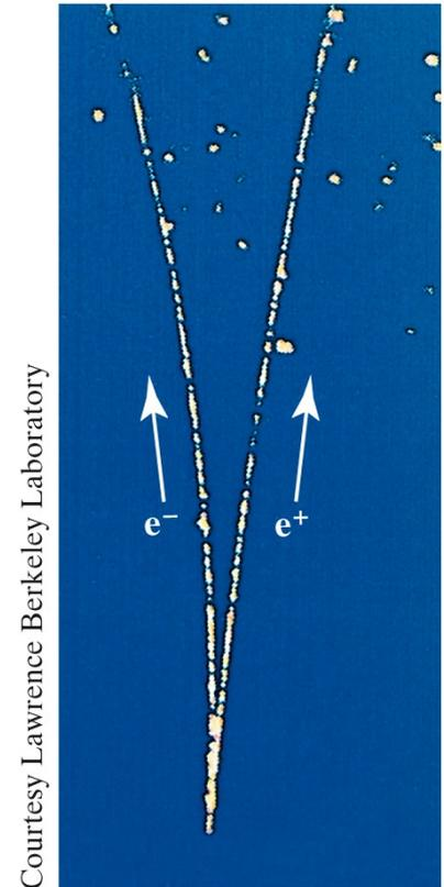
A photograph of trails of bubbles left in a bubble chamber by an electron and a positron. The pair of particles was produced by a gamma ray that entered the chamber directly from the bottom. Being electrically neutral, the gamma ray did not generate a telltale trail of bubbles along its path, as the electron and positron did.
