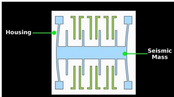
Figure 3: The accelerometer in a mobile phone uses the capacitance measurement to infer a change in position of the seismic mass. The two plates are colored blue and green. From Ref 5.
