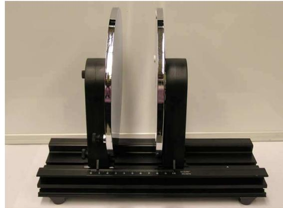
Figure 2: A parallel-plate capacitor in which the plate spacing is variable. From Ref 4.
