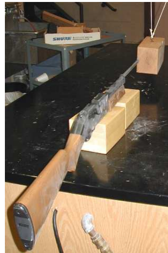
Figure 2: A ballistic pendulum is used to measure the muzzle velocity of a BB. The collision between the BB and the wood block is completely inelastic. Kinetic energy is not conserved, but momentum is conserved. From Ref 3.
