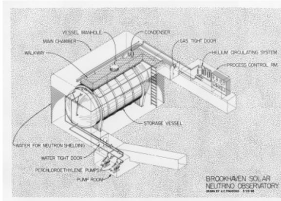
Water tank shielding
