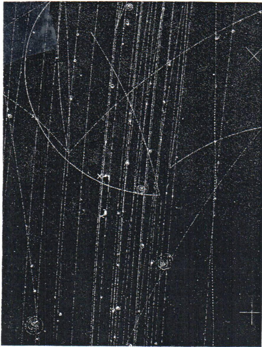
Figure 1.3 An example of associated production, due to the interaction at A of a 4\text{-GeV}/c negative pion in a hydrogen bubble chamber: \pi^- + p \rightarrow \Lambda + K^0 . The \Lambda -hyperon decays at B according to \Lambda \rightarrow p + \pi^- , and the K^0 -meson at C according to K^0 \rightarrow \pi^+ + \pi^- . (Courtesy CERN.)
