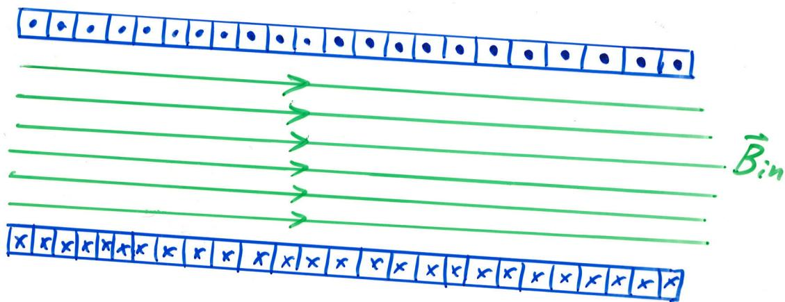
Magnetic field inside a solenoid by Ampere's Law:  $n$  turns of wire per unit length
