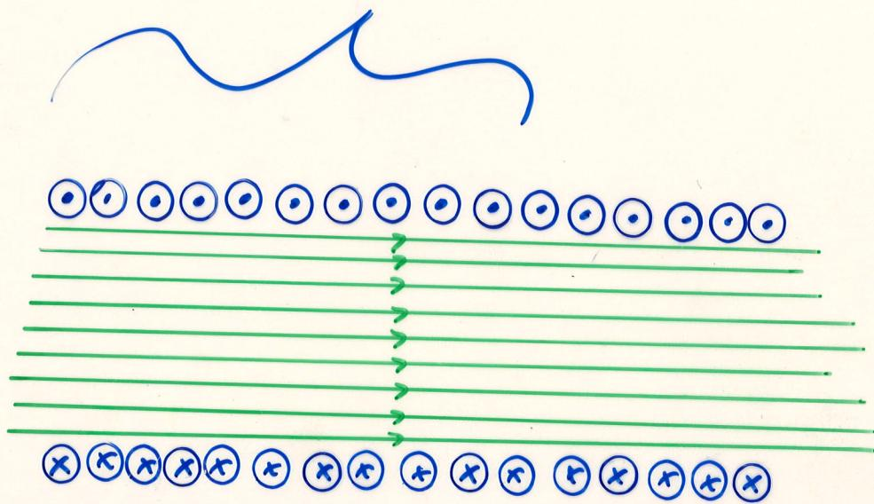
If the solenoid is very long compared to its radius and if the coils are closely spaced then:
