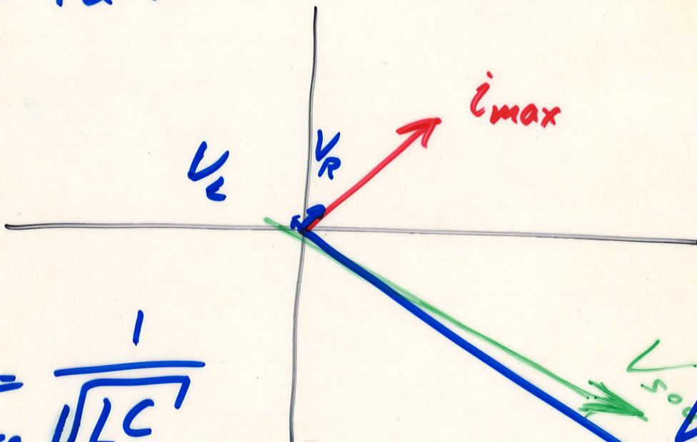
$$\begin{aligned} \omega_{\text{Resonance}} &= \frac{1}{\sqrt{LC}} \\ &= \frac{1}{\sqrt{4 \mu H \cdot 10 \mu F}} = \frac{158,000}{\frac{\text{rad}}{\text{s}}} \text{ rad/s} \end{aligned}$$
