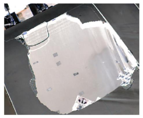
Foam impact experiment, at speeds estimated from video of strike on actual shuttle. Resulting damage. Piece hitting Columbia was 400 times bigger than any previous observed strike – outside experience of foam strike models.
