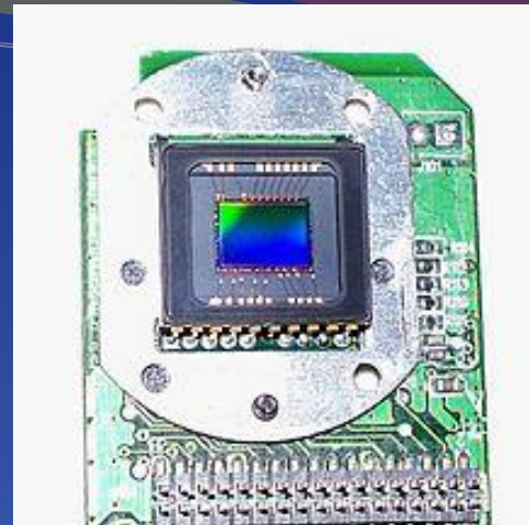
CCD from a 2.1 megapixel Hewlett-Packard digital camera.
