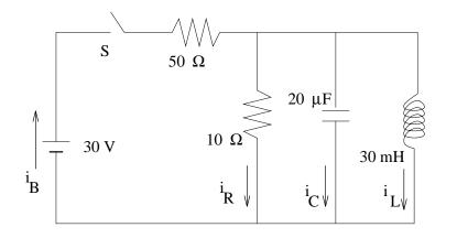
What are the four currents an instant after the switch is closed? (Positve values if the currents are flowing in the directions indicated; negative if flowing the opposite direction.)
