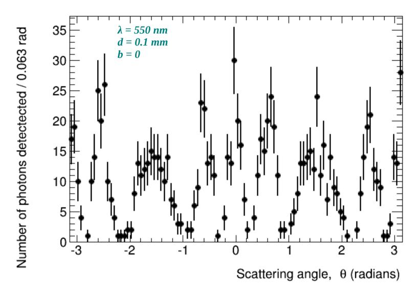
1000 simulated photons scattered through a double-slit experiment. This was done in C++ using the free ROOT High-Energy Physics data analysis framework, so I could easily generate a *histogram* – a binned data sample.
