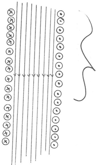
If the solenoid is very long compared to its radius and if the coils are closely spaced then:
