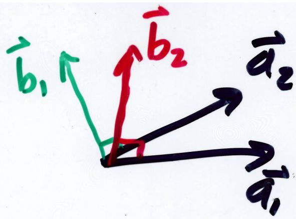
$$\vec{b}_1 = \frac{2\pi \vec{a}_2 \times \vec{a}_3}{\vec{a}_1 \cdot (\vec{a}_2 \times \vec{a}_3)}$$
