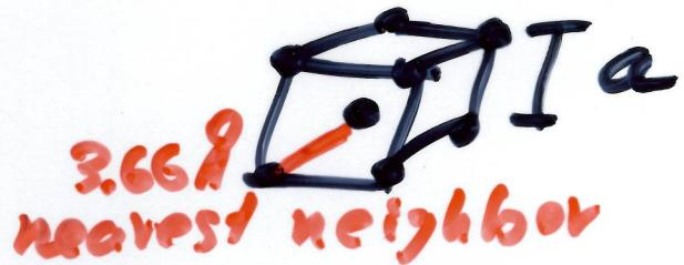
For Na, bcc - 2 atoms / non primitive cubic cell
