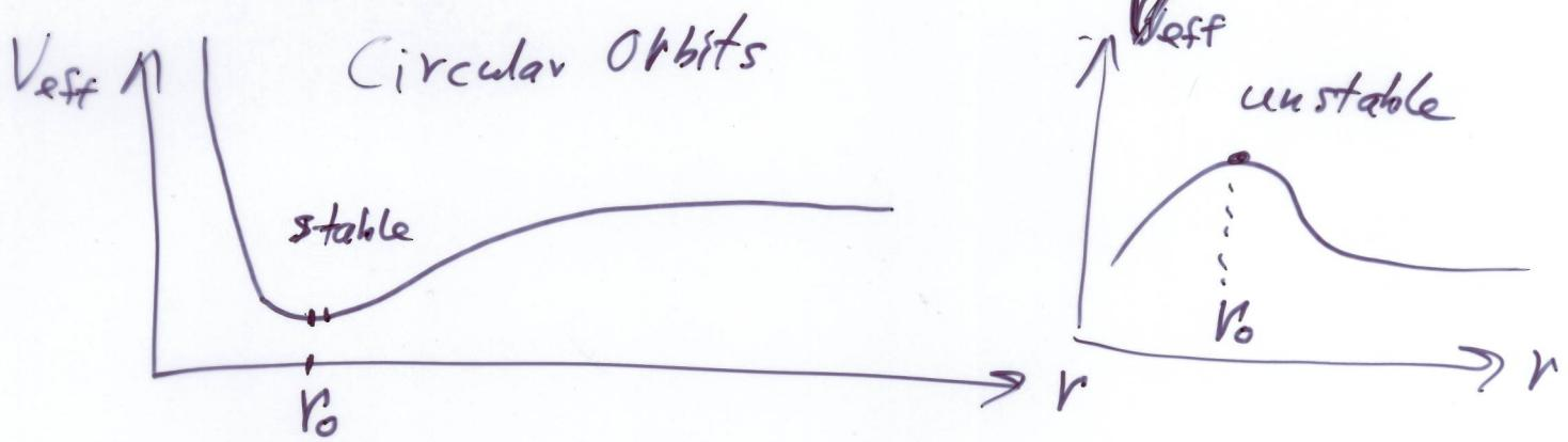
$$\text{If } r = r_0 \Rightarrow \dot{r} = 0, \ddot{r} = 0 \Rightarrow f(r_0) = -\frac{\ell^2}{mr_0^3}$$
