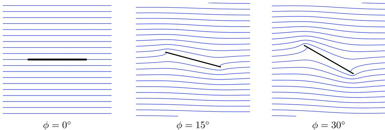
**Figure 7.30.** Fluid Flow Past a Tilted Plate.
