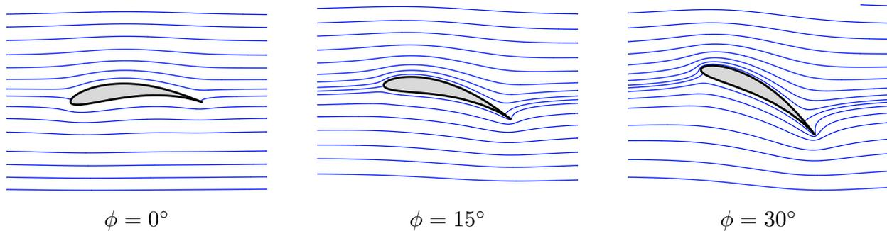
**Figure 7.31.** Flow Past a Tilted Airfoil.
