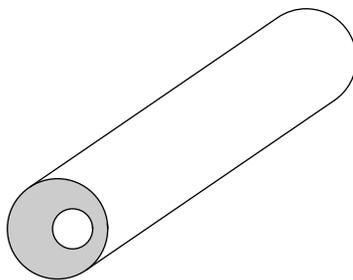
**Figure 7.26.** A Non-Coaxial Cable.
