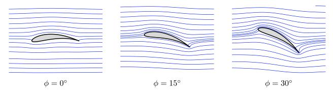
Figure 7.31. Flow Past a Tilted Airfoil.
