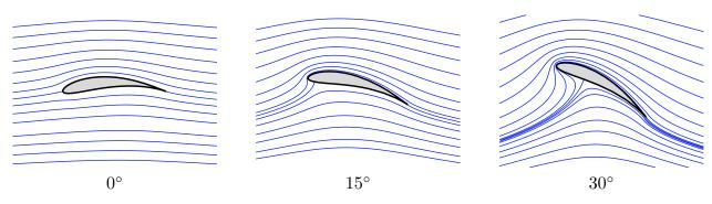
Figure 7.37. Kutta Flow Past a Tilted Airfoil.
