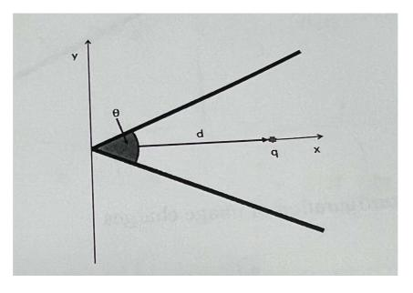
Two perfectly conducting infinite and grounded half-planes intersect at an angle  $\pi/3$  radians. A charge q is located halfway between the planes at a distance d from the intersection. Find the potential energy of the configuration.
