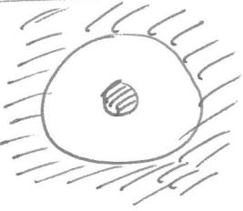
can support a TEM wave by placing a potential difference between the two conductors. Then find
