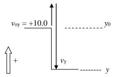
$a_y = -9.80 \text{ m/s}^2$   $y - y_0 = -100 \text{ m}$  (change in y)  $v_y$  velocity just before impact speed is  $|v_y|$
