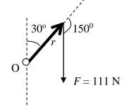
$\underline{\mathbf{F}}$  applied at  $\underline{\mathbf{r}}$  produces a clockwise torque about O
