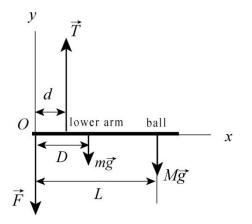
$\vec{T}$  = biceps muscle tension (required)  $\vec{F}$  = tension in elbow joint (required)  $m\vec{g}$  = 1.8 x 9.8 = 17.64 N  $M\vec{g}$  = 7.2 x 9.8 = 70.56 N D = 0.15 m d = 0.04 m L = 0.33 m
