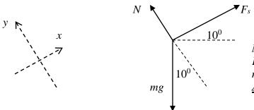
N = normal force magnitude (unknown)  $F_s$  = static friction magnitude (unknown) mg = gravity magnitude =2.0x9.8=19.6 N <u> $\Delta r$ </u> in x direction
