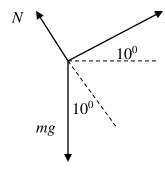
N = normal force magnitude (unknown)  $F_s$  = static friction magnitude (unknown) mg = gravity magnitude =2.0x9.8=19.6 N  $\Delta r$  in x direction
