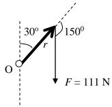
**<u>F</u>** applied at <u>**r**</u> produces a clockwise torque about O
