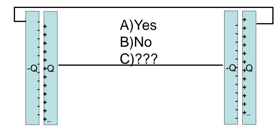
Two very strong (big C) ideal capacitors are well separated. What if they are connected by one thin conducting wire, is this electrostatic situation physically stable?
