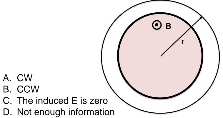
The current in an infinite solenoid with uniform magnetic field **B** inside is increasing so that the magnitude B in increasing with time as  $B=B_0+kt$ . A small circular loop of radius r is placed outside the solenoid as shown. What is the emf around the small loop?
