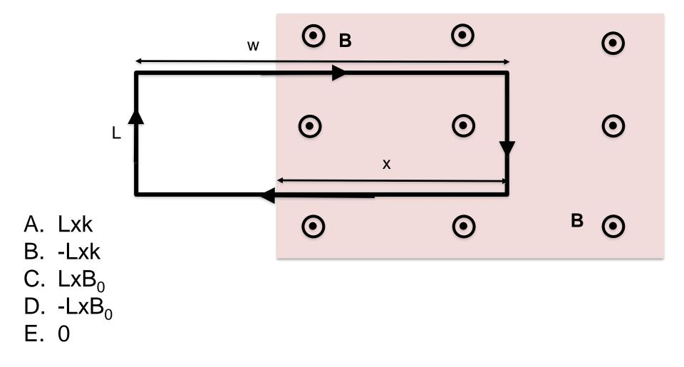
One end of stationary rectangular metal loop is in a region of uniform magnetic field **B**, which has magnitude B increasing with time as  $B=B_0+kt$ . What is the direction of the field **B**<sub>ind</sub> created by the induced current in the loop, in the plane region inside the loop?
