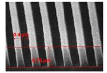
A close-up of a diffraction grating, consisting of a large number of small slits. Like the double-slit case, each slit causes diffraction and then the diffracted light from each slit can interfere on an observation screen. A diffraction grating is better than 2 slits because it lets more light through, making observation easier.
