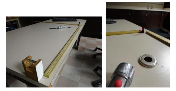
Place two meter sticks on the table in an L-shape, with the metric scale up. Have one end of one stick be near the table edge (this is where the grating will go to make observation easier). These meter sticks form the sides of a right-angled triangle that can be used to calculate the angles of diffraction  $\theta$ .
